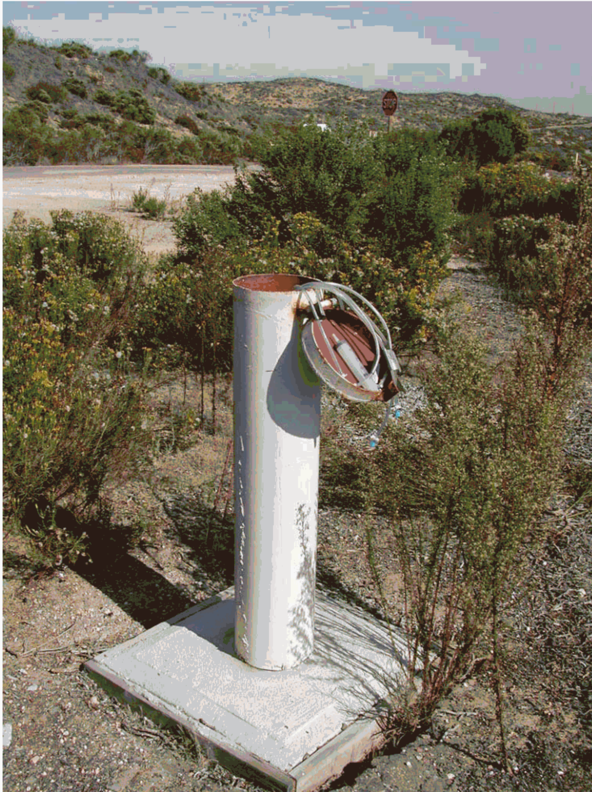
Figure C-3. Vertically-nested soil-gas-sampling probes sealed at the ground surface with a concrete pad and a vertical surface casing.
